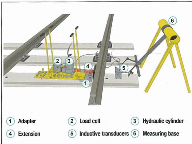
Fig. 1: Test set-up for LTR field measurement as adopted by the Institute of Road, Railway and Airfield Construction of TUM
