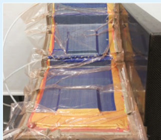
The gelcoat/infusion part ready for the resin infusion process to commence
