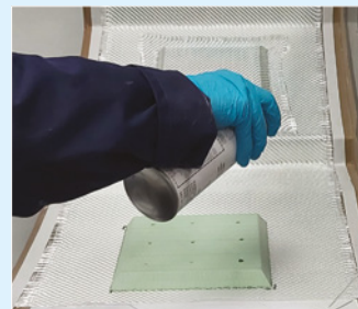
Spray adhesive required for manufacture of the gelcoat/infused part
