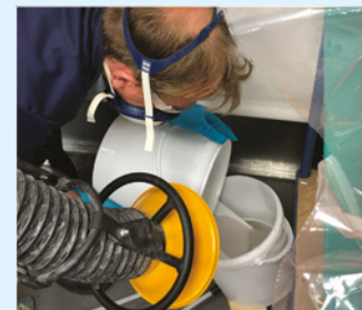
Resin has to be weighed, mixed and the part infused before cure and postcure
