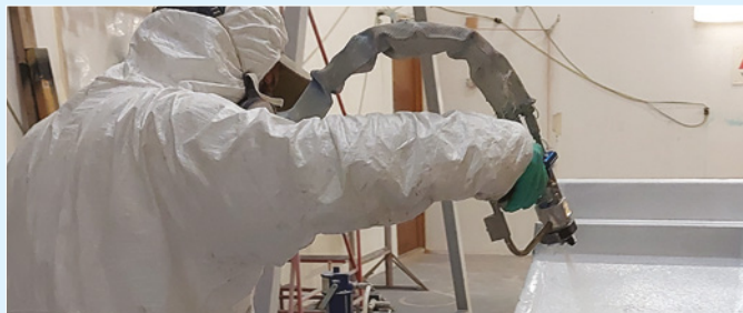
Infusion Solution: Spraying the gelcoat into the mould – additional PPE and preparation time is necessary
