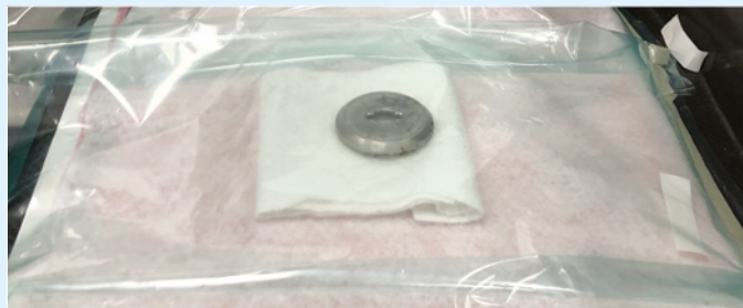
Applying vacuum consumables to SPRINT™ part, after which it's ready to cure
