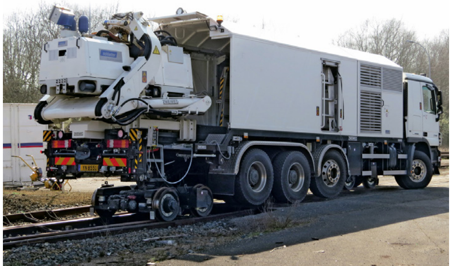
Supra Roadflex – AMS200 rail welding machine
