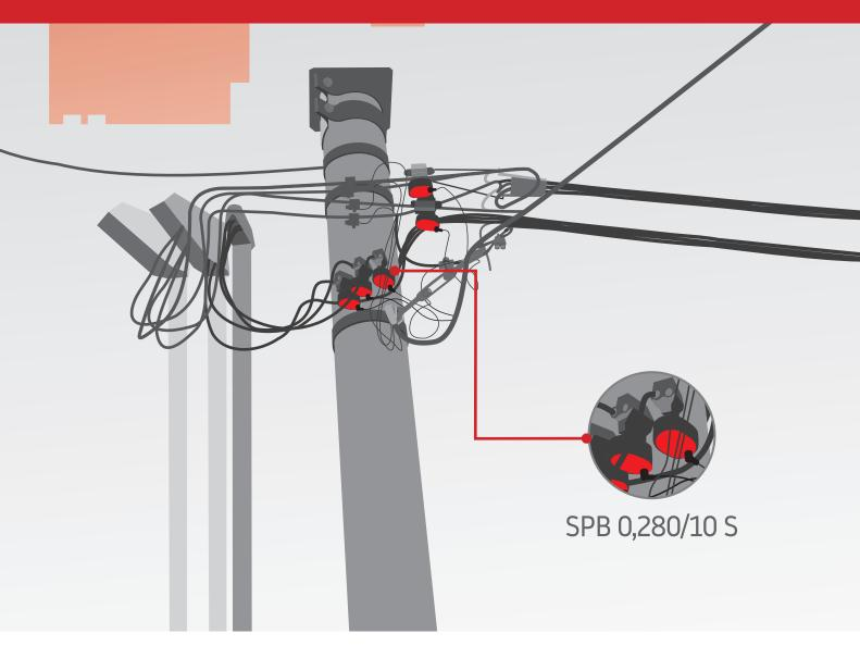
SPB \*/10 PP\* - on flat busbars SPB \*/10 AlFe\* - on bare overhead conductors SPB \*/10 S\* - on insulated overhead conductors
