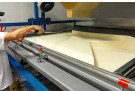
Thermoformed (Vacuum Formed) Interior Panels
