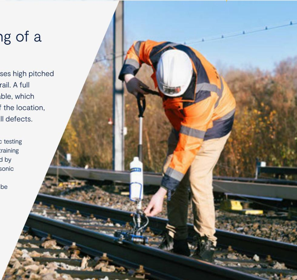
Ultrasonic Testing device
