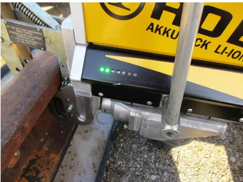
**Fig.5:** Electronically supported work: The LED display of the battery powered rail drilling machine shows the manual feed rate.
