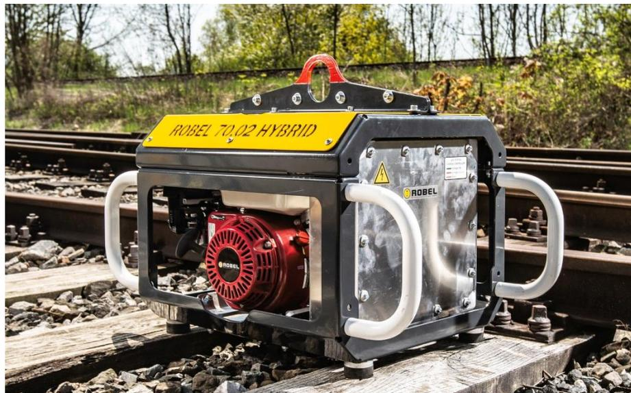
**Fig.8:** Portable solution: A separate Powerpack supplies the ROGRIND HF Head high-frequency grinding machine.
