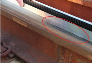
Fig. 4: Dents caused by wear in the annealing zone of a thermite weld Source: ÖBB
