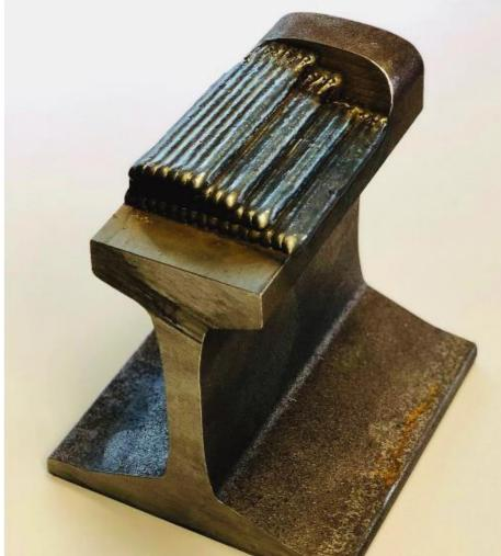
Fig. 6: Instead of replacing parts, the original geometry is reconstructed quickly in layers and thus completely reinstated. Source: ROBEL Bahnbaumaschinen GmbH
