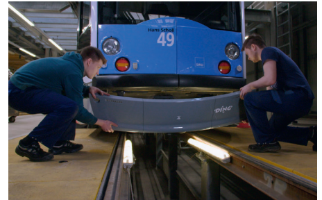
Installation of the 3D printed housing cover
