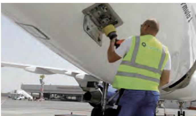
The underground pit system follows the international standards (IATA, ACI) and supports the industry with innovative solutions by providing savings, extra revenues and reducing pollution from aviation. The pop-up pits are located at a minimum distance from aircraft connections points in order to improve system performance and ensure the functionality of all systems.
