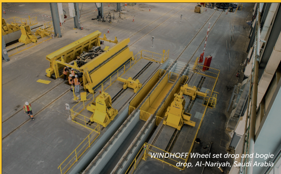
The mobile wheelset rotating device supports visual inspections
