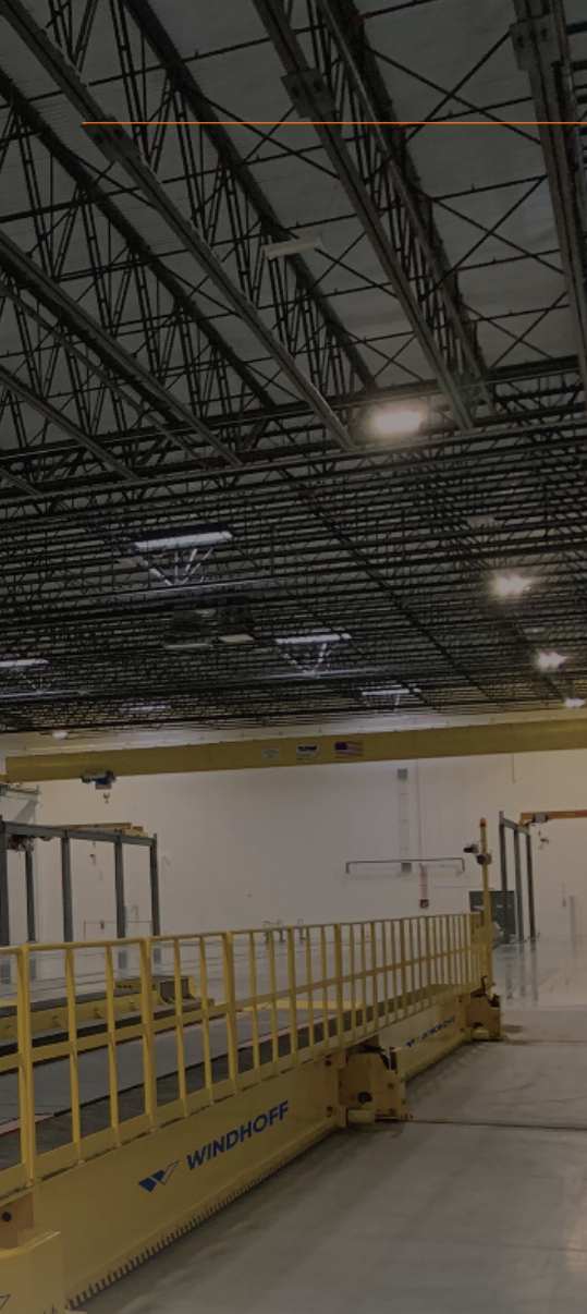
Traverser: Pitless Design, Double Track 2 x 65 tons, CRRC Chicago, USA
