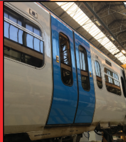
Doors with No Delamination or Corrosion
