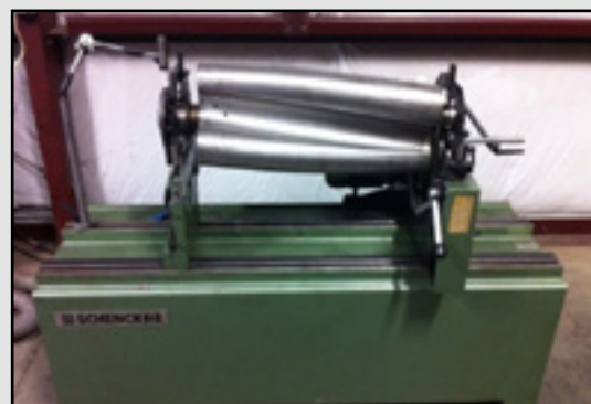
All Scrolls Are Precision Balanced
