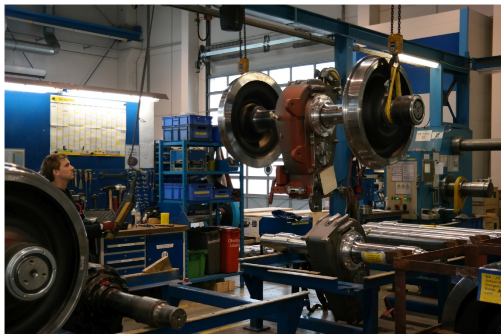
Fig. 3: Overhaul of a wheelset with axle gearbox
