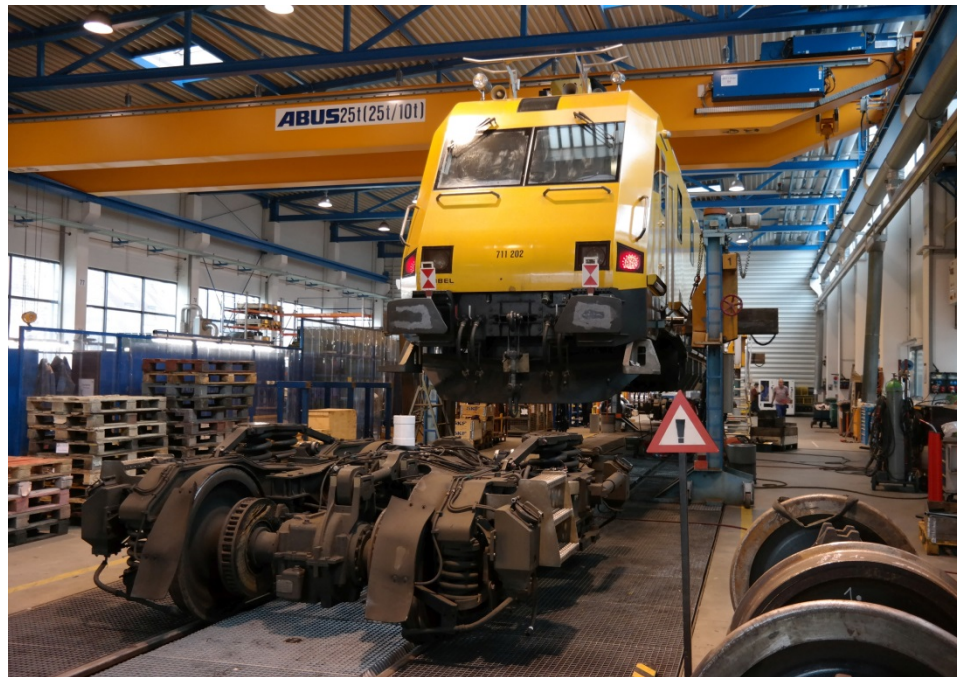
Fig. 6: Dismantling the old bogie during an overhaul
