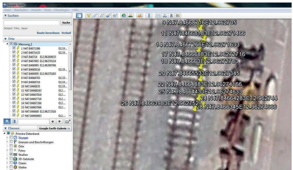
Fig. 8: Transferring the recorded GPS data onto Google Maps facilitates locating possible faults in track screw joints.
