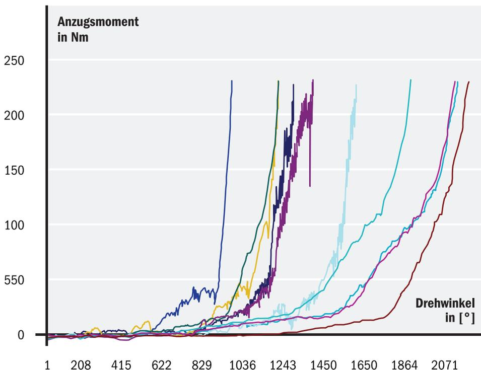
Fig. 2: Torque versus angle of rotation of various nuts on K track. The left-hand curves show hard screw joints; every type of lubrication shifts the curves to the right. Graphs recorded with ROBEL servo wrench.
