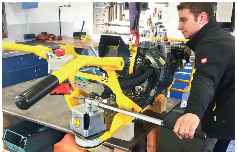
Fig. 4: The annual calibration is carried out by trained staff of the contractor using the torque measurement unit.
