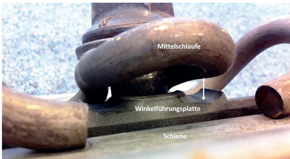
Fig. 1: The geometric nominal tensioning for W track is  $\leq 0.5$  mm as per DB Guideline 824.5050.
