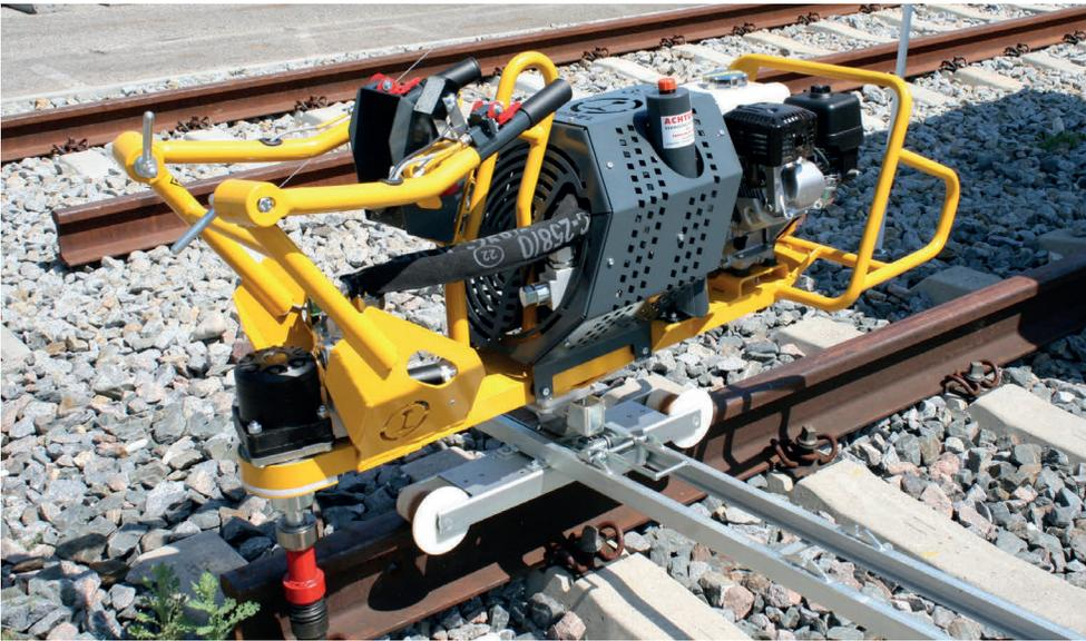
Fig. 5: With the handles folded in, the wrench can be transported easily by four people, even if space is tight.
