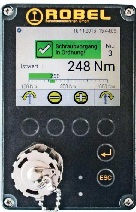
Fig. 6: The PLC display shows that the wrenching process has been completed in line with the guideline.
