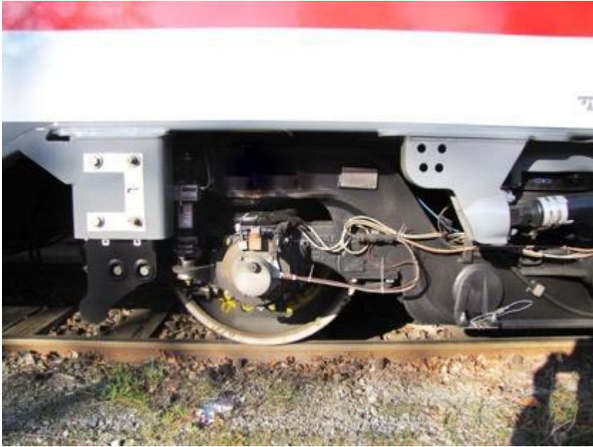
For the measurements, the ASC sensors are mounted on the wheelsets of the trains Photo: Alstom
