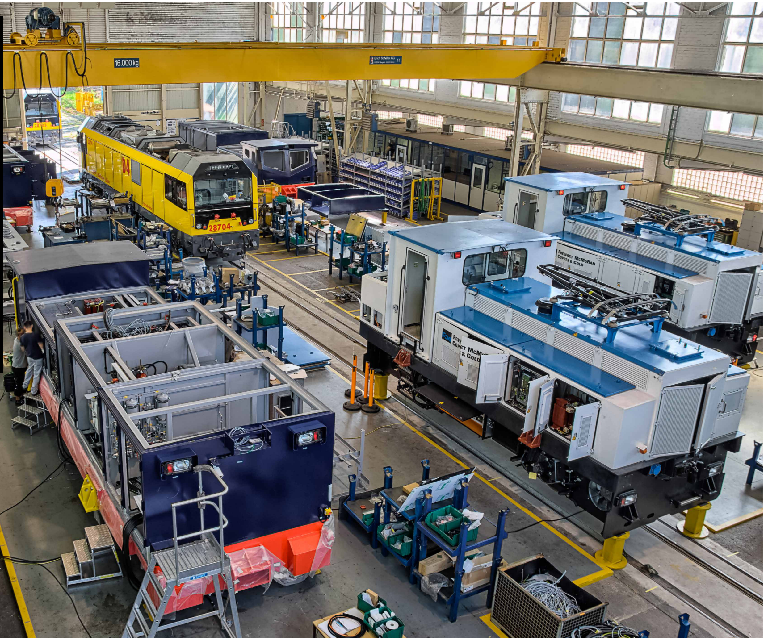
Working to capacity: various types of locomotive are built simultaneously in the Schalke assembly building.
