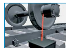
Positioning in the hot box detection systems
