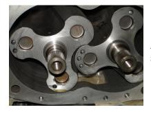
All Roots Blower scrolls are remanufactured and balanced prior to installation.
