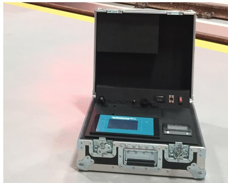
The PTW indicator provides instant weighing results via printout or CSV file. Operating via three main screens the robust and IP65 rated indicator provides easy to use functions and immediate weighing information.
