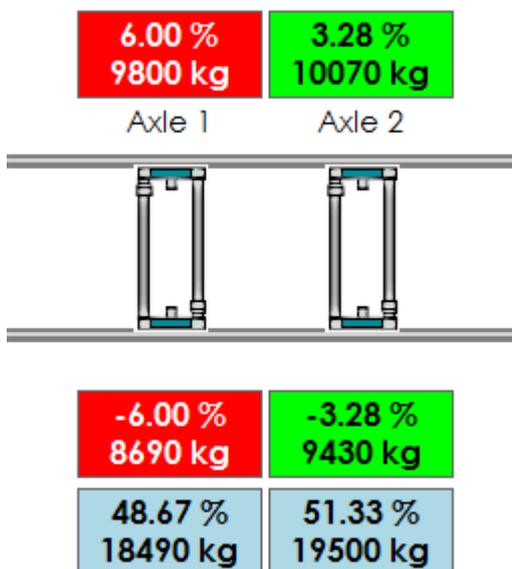
Our intuitive, multilingual ptwX train weighing software is designed and developed in-house and provides real time 'live' displays. Multiple customisations such as weighing units and information on weight differentials are also available
