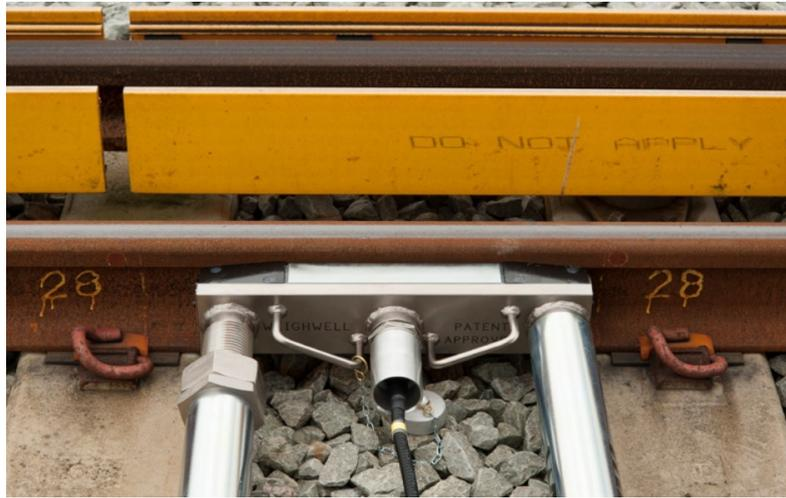
Our PTW allows for greater flexibility without the need to remove rail fastenings due to its length of only 500mm. This results in a more convenient installation and less 'flexing' of the system. The benefits of this are more accurate, repeatable and reliable weighing results.
