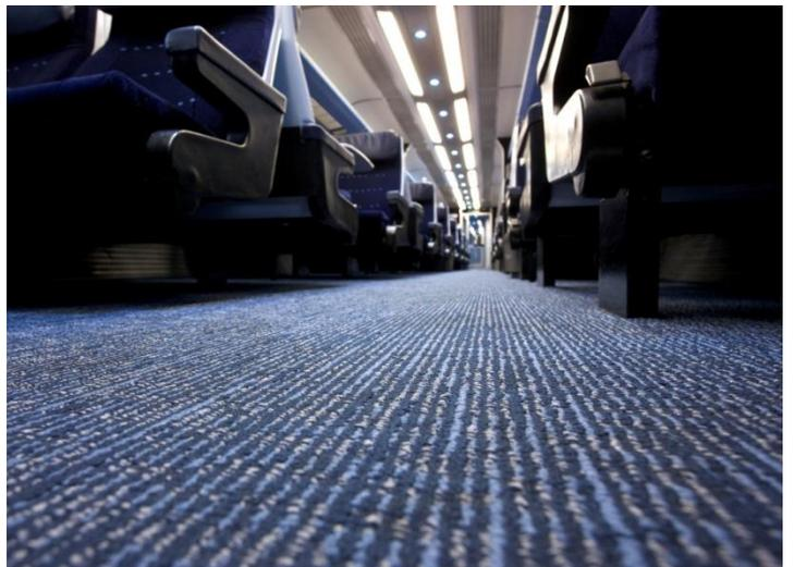
Two products that are proving to be right on track with East Midlands Trains are Tessera Alignment FR carpet and Coral Brush Activ FR entrance flooring from Forbo Flooring Systems. The operator recently completed the refurbishment of its entire HST fleet at its Neville Hill depot in Leeds and fitted these two high performance Forbo textile floor coverings throughout 93 saloon carriages during the programme.
