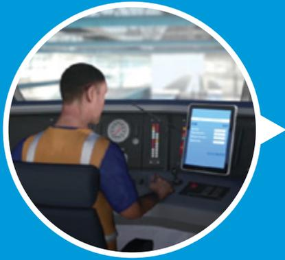
The **Trimble® CAB advisory system** is an on-board solution that informs the driver about train performance and adherence to timetable.
