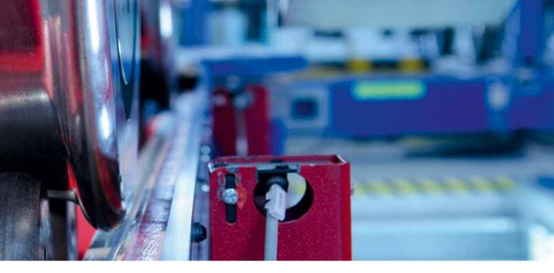
Precision is needed in the workshops to ensure that trains can run quickly and safely with minimum wear. Here bogies and rail car bodies are measured, adjusted and thereby optimised under simulated load conditions, both when originally built and when undergoing maintenance.
