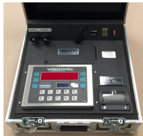
Digital indicator and printer in robust carry case.
