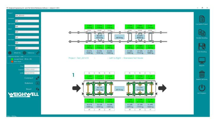
Our intuitive, multilingual ptwX software is designed and developed in-house and provides real time 'live' displays. Multiple customisations such as weighing units and information on weight differentials are also available. Our easy to use software also allows for fully customised reporting options to be selected with the ability for reports to be exported in standard formats such as pdf and csv.
