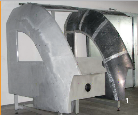
1 Front module of railway vehicle made of aluminum foam sandwiches with aluminum cover sheets
