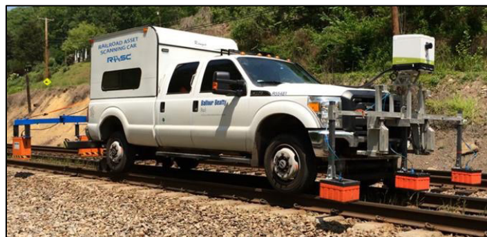
Figure 2: RASC® solution deployed from hy-rail vehicle on the CN network.
