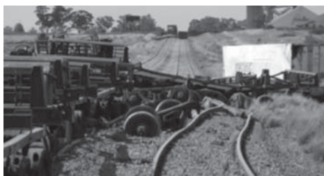
Australia: Undetected weakness in the track formation. Dip in track and adverse twist caused bogie to derail.
