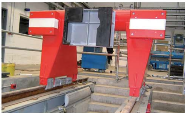
Type 6 EB Friction Buffer Stop Special design for work shop tracks Installation location: Northampton, Great Britain
