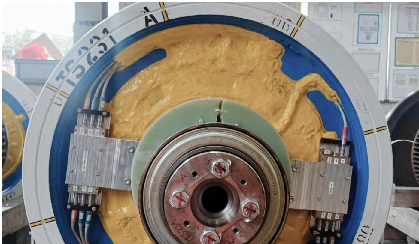
imc MTP-NT-XS Telemetry System in a road test, installed on a wheel set ©TÜV SÜD Rail
