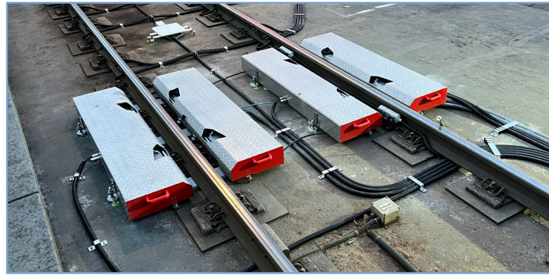
Automated 3D Wheel Measurement System: Laser scanning technology captures precise wheel profiles and wheel diameter without stopping the vehicle
