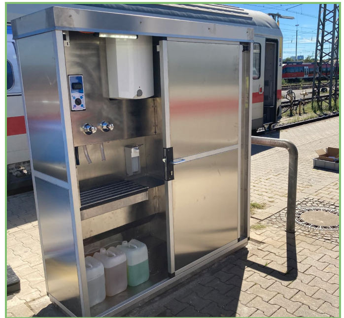
Stainless Steel Cabinet with self-closing sliding doors in Dortmund, Germany (DB)
