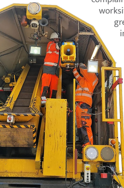
Left image: Warning devices can be installed directly on the construction machines which places the warning signal exactly where the work is carried out
