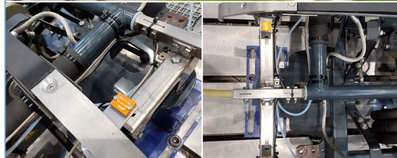
ASC 4421MF accelerometer used in pantograph testing at 350+ km/h © ASC Sensors
