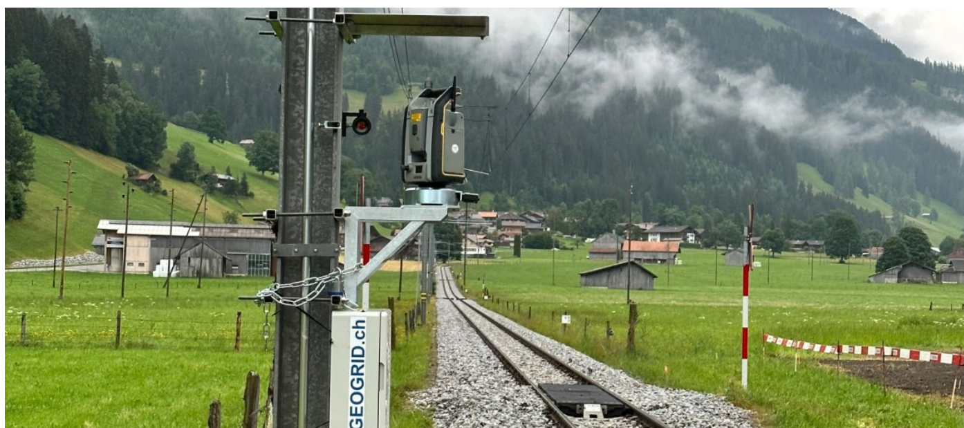
A visual of a mounted Trimble S9 total station next to a railway track for GEOGRID AG project © GEOGRID AG
