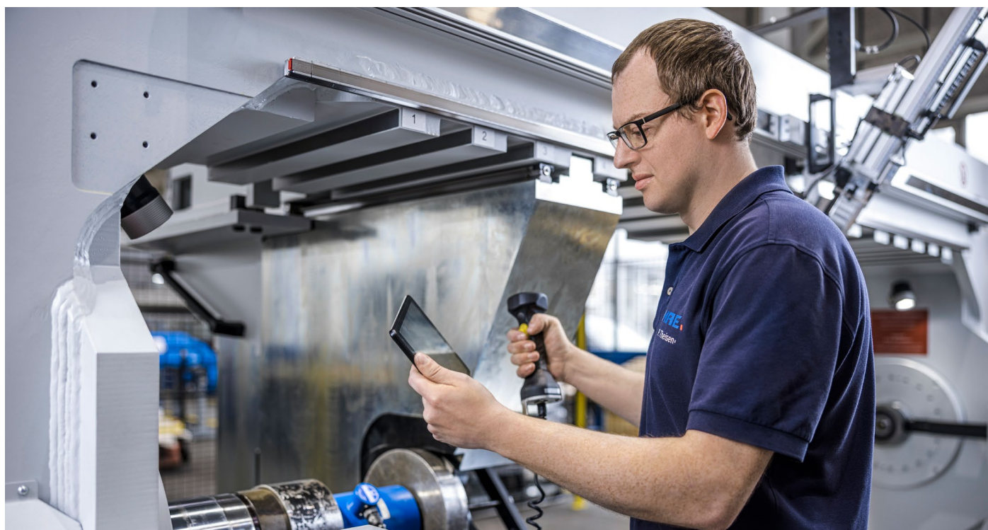
MAE technician during calibration of a wheelset press
