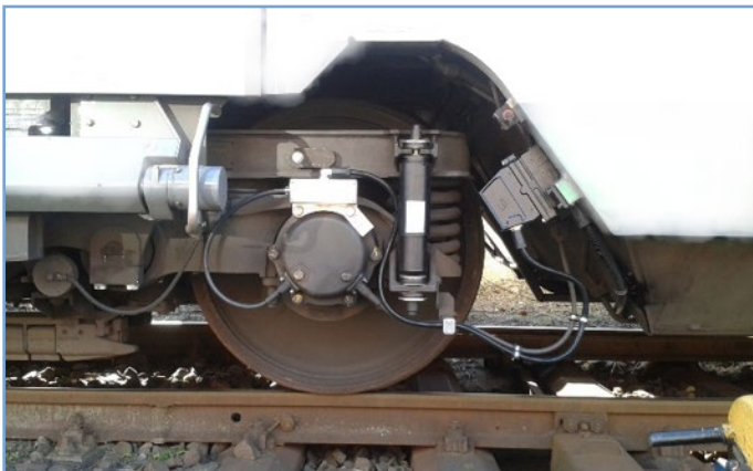
Installed DB Systemtechnik sensorbox mounted on the wheelset
