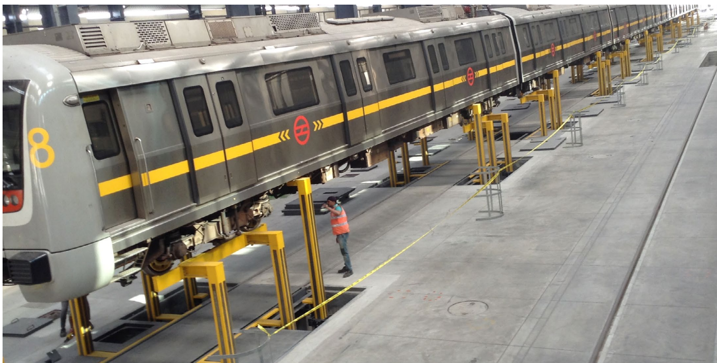
Example of a project that has already been completed: an 8-carriage system at the Badli depot in New Delhi
