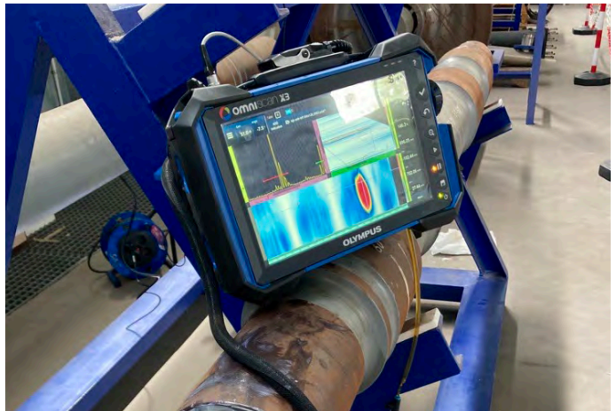
Deployment of the scanner and probe with OmniScan™ X3
