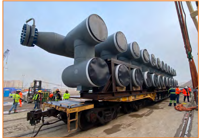
The cargo was railed from Kansas to Texas using a 70' 8-axle railcar
