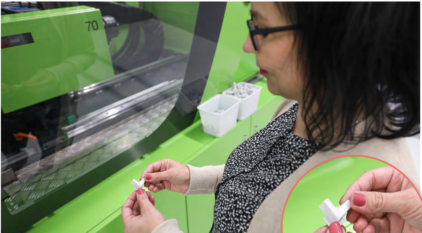
A moulded corner part made of light grey silicone. “This is a fine example of a combined solution. Four corners like this and extruded silicone profiles will form a sealing frame solution for our customer,” Laihonen says
