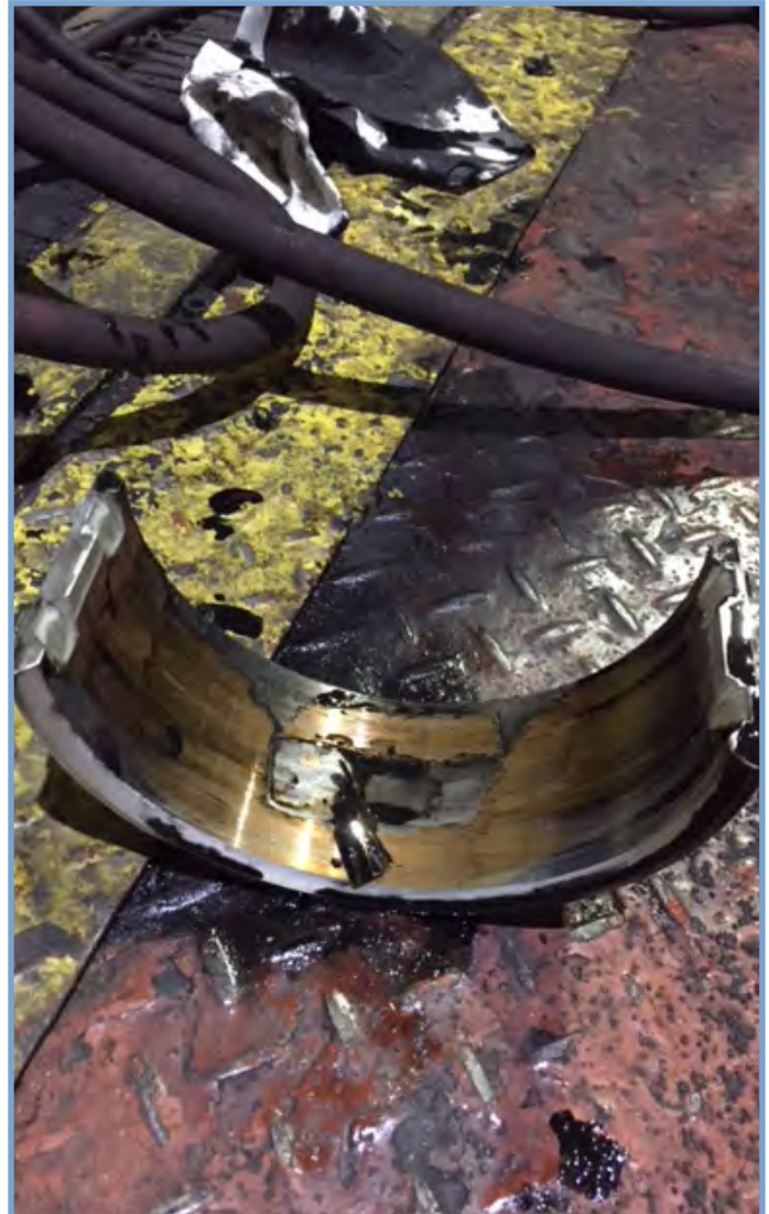
Shattered main bearing
