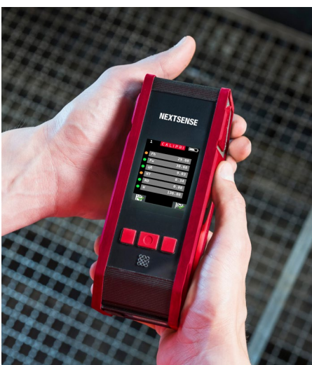
Figure 3: Colour-coded measured variables on the sensor
