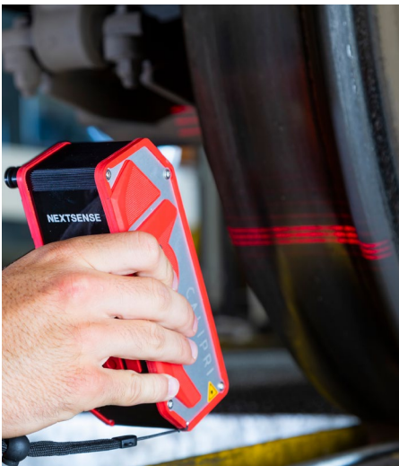
Figure 2: Contact-free measurement of the wheel profile
