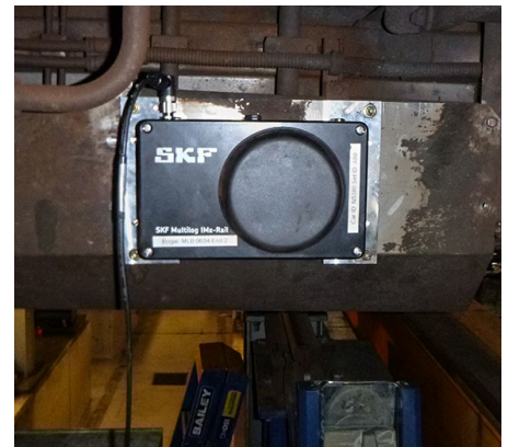
SKF's advanced multilog on-line system IMx-Rail for increased rail traffic reliability
