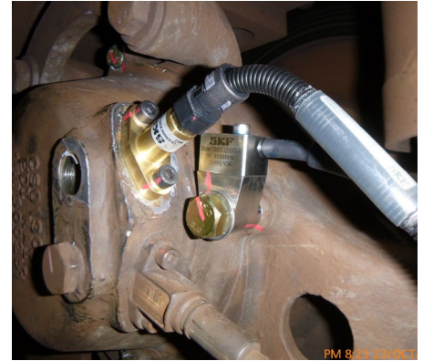
SKF's speed and vibration sensor mounted on axlebox
