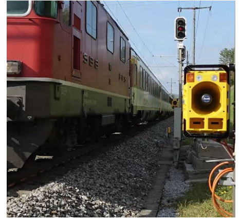
Image 3 ZPW126-31 mounted using magnet fastening
