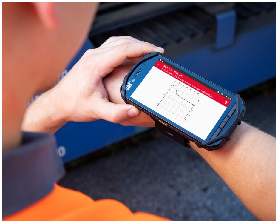
Figure 5: View of the wheel profile as point curve
