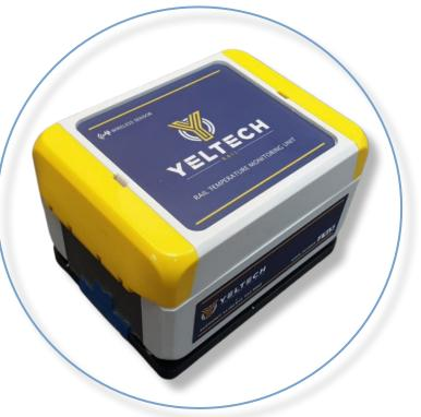
Normal rate is when the RTMU wakes up and sees the temperature below 25°C, it will store the data and then send the bulk of readings/data every 12 hours. Fast rate of the RTMU is when the temperature exceeds the threshold of 25°C and the CRT alarm thresholds that have been set. When the RTMU wakes up, if the temperature is above 25°C, then it will keep transmitting data to the server every 30/60 minutes.
