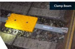
Originally designed for the installation of TPWS (Train Protection & Warning System) in the UK, the Balise Mount System (BMS) comprises a GRP beam with stainless steel yokes that use the existing rail fastenings or the rail foot to hold the beam in track. The BMS allows for very quick installation and removal of devices from track, typically taking less than 2 minutes.
