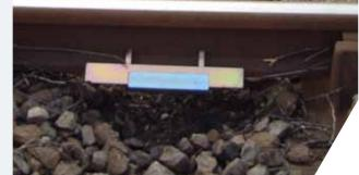
Robust, lightweight Temporary AWS magnets that can be quickly and easily installed where there is a need to place an emergency or temporary speed restriction. The magnets are available in standard strength (yellow) and extra strength (green for third rail applications).
