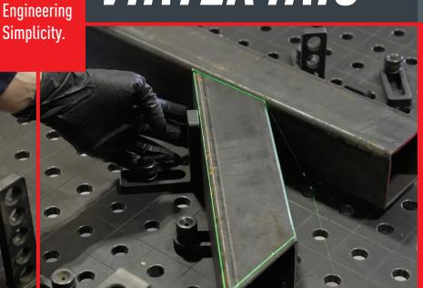
Virtek Iris™ 3D simplifies fitting and accelerates the assembly process by eliminating manual measurement, marking and templates.
