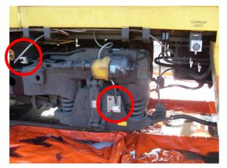
Figure 8 : QRN 5000 Locomotive shown with V/TI Monitor Axle Sensors
