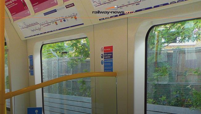
The Glasgow Subway order represents the first time Stadler has supplied trains for a driverless underground metro system. The design of the train also differs as they need to fit a track gauge of 1,219 mm and tunnels that are just 3.4 metres in diameter. While the new trains are the same length as the vehicles they will be replacing, they are four cars long rather than three.
