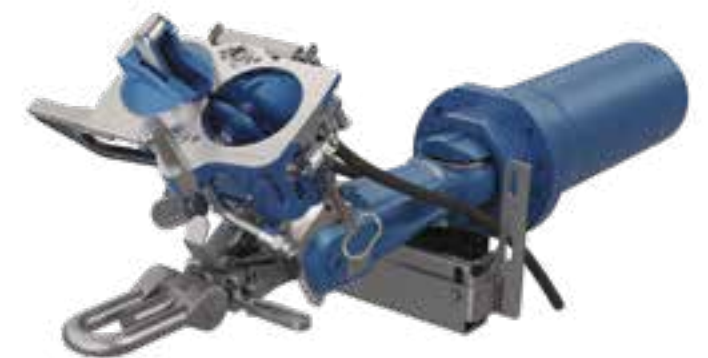
HYBRID DAC FOR LOCOMOTIVES SCREW COUPLER MODE
