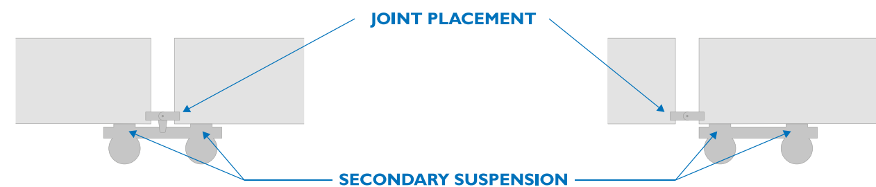
FIGURE 1. JACOB'S BOGIE AND SEMI-TRAILER JOINT.
