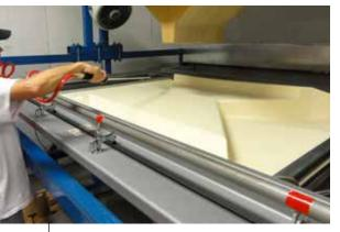
Thermoformed (Vacuum Formed) Interior Panels
