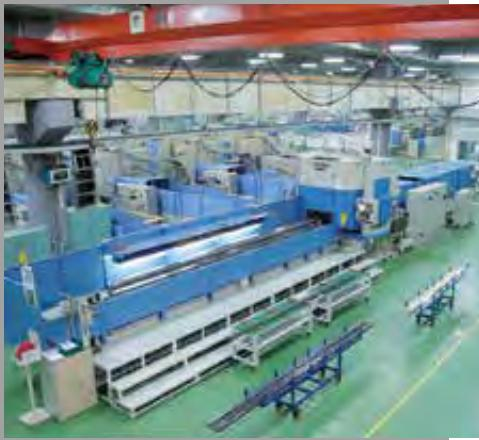
7-meter grinding machine for LM rails
