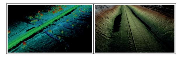
Integrated data views are available through the RASC® Viewer desktop software solution. This links the CTQI metric (and all of its components), laser views, and track geometry, to on-track video data and Google Map overlays, referenced by milepost or kilometre post and latitude/longitude.
