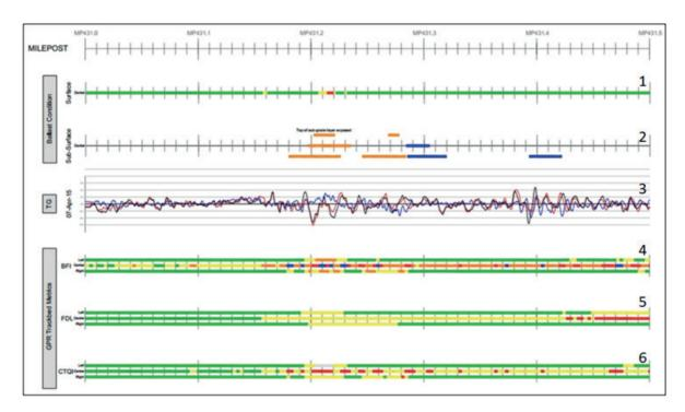
The above example shows an integrated track chart view for a 0.5mile section of track presenting mapped surface mud spots (1), below-ground extent of mud spots and ballast pockets (2), track geometry - left/right profile and twist (3), ballast fouling index (4), ballast fouling depth (5) and CTQI (6).
