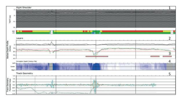
RASC® data can also provide valuable input to monitor settlement of trackbed on embankments following heavy rainfall events and can be used to map sand ingress in and around ballasted track following sand storms in desert areas.
