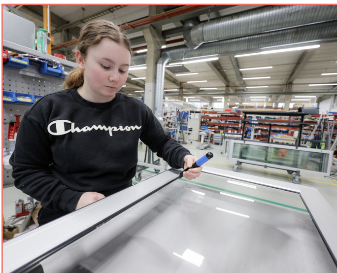
Polarteknik’s employee installing a window seal frame
