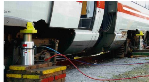
Jacking and skidding used for heaviest rail cars
