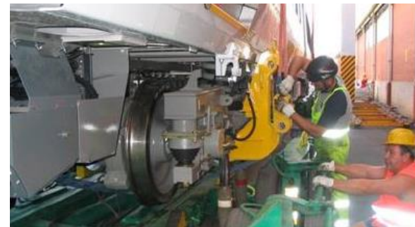
Positioning lifting shoes on the car (client-specific)
