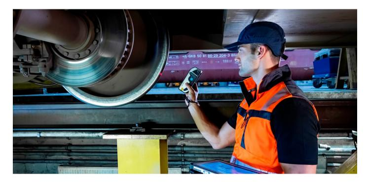
NEXTSENSE's Team Leader Railway Applications. "There are a wide variety of measurement modules to choose from. These set the measurement parameters for the sensor, which can then be guided around the wheel to gather the necessary data.
