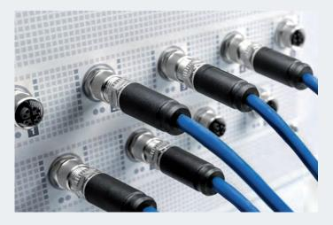
As 8-pole, X-coded compact connectors in Cat. $6_{A'}$ , the M12 from Telegärtner can transmit data rates of up to 10 Gbit/s in accordance with IEC 61076-2-109:2014. Even in harsh environments, the high bandwidth is ensured by separating the four pairs with a cross shield (X-coding). Remote powering of end devices is also possible.
