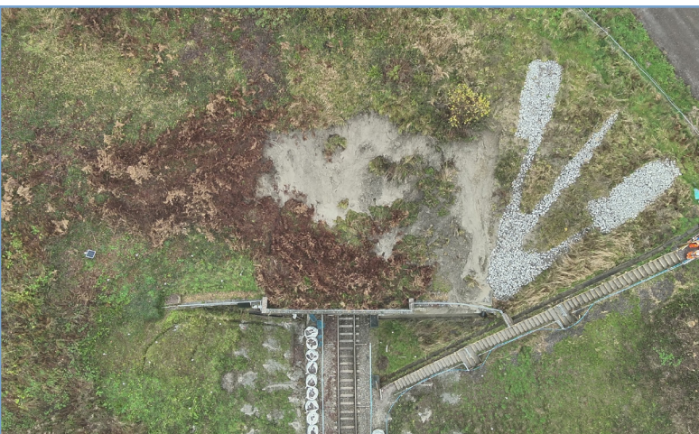
Figure 2: Wireless monitoring is routinely used by Network Rail for early warning of slope failures such as this one at Crewkerne, Somerset
